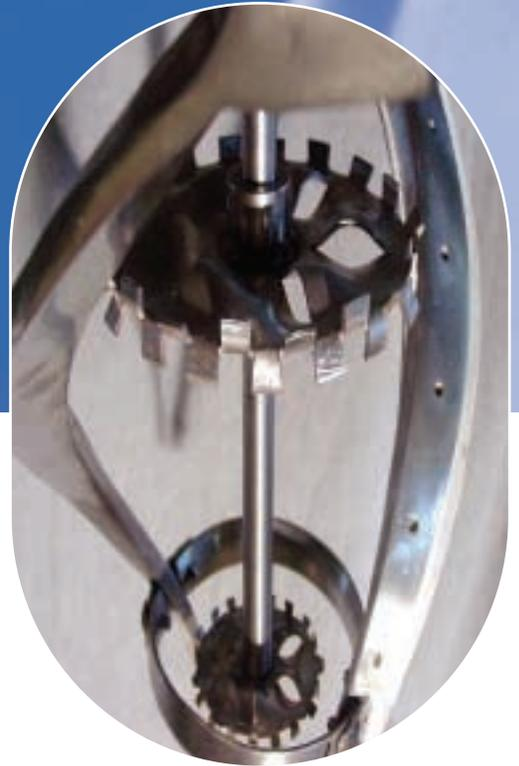
The **SC Mixer** is ideally suited for mixing or drying applications that require *finite control of reaction kinetics*. With either adjustable or high shear capabilities, this mixer routinely handles materials with a viscosity as high as 3 million Centipoise.
